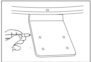
7. Clean roof area where the base feet will be attached to the roof. Do not erase your marks!
